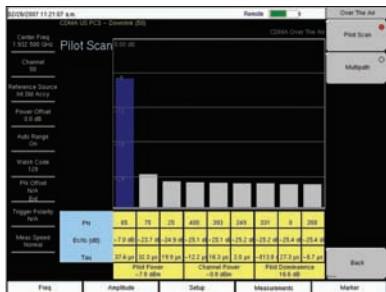
CDMA Over the Air measurement display
