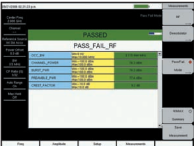
Using Master Software Tools create and download custom Fixed WiMAX Pass/Fail test sets.
